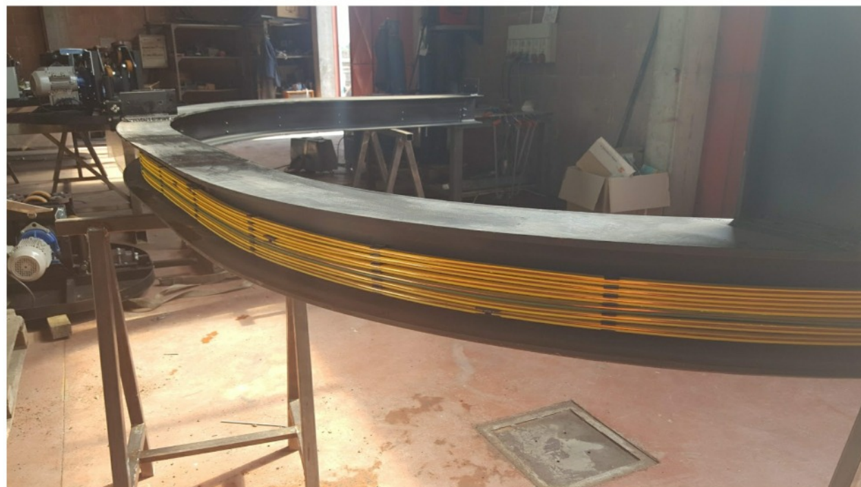
Manufacturing of the rail in IPN
